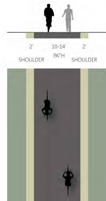
Figure A-8: Preferred Path Dimensions
