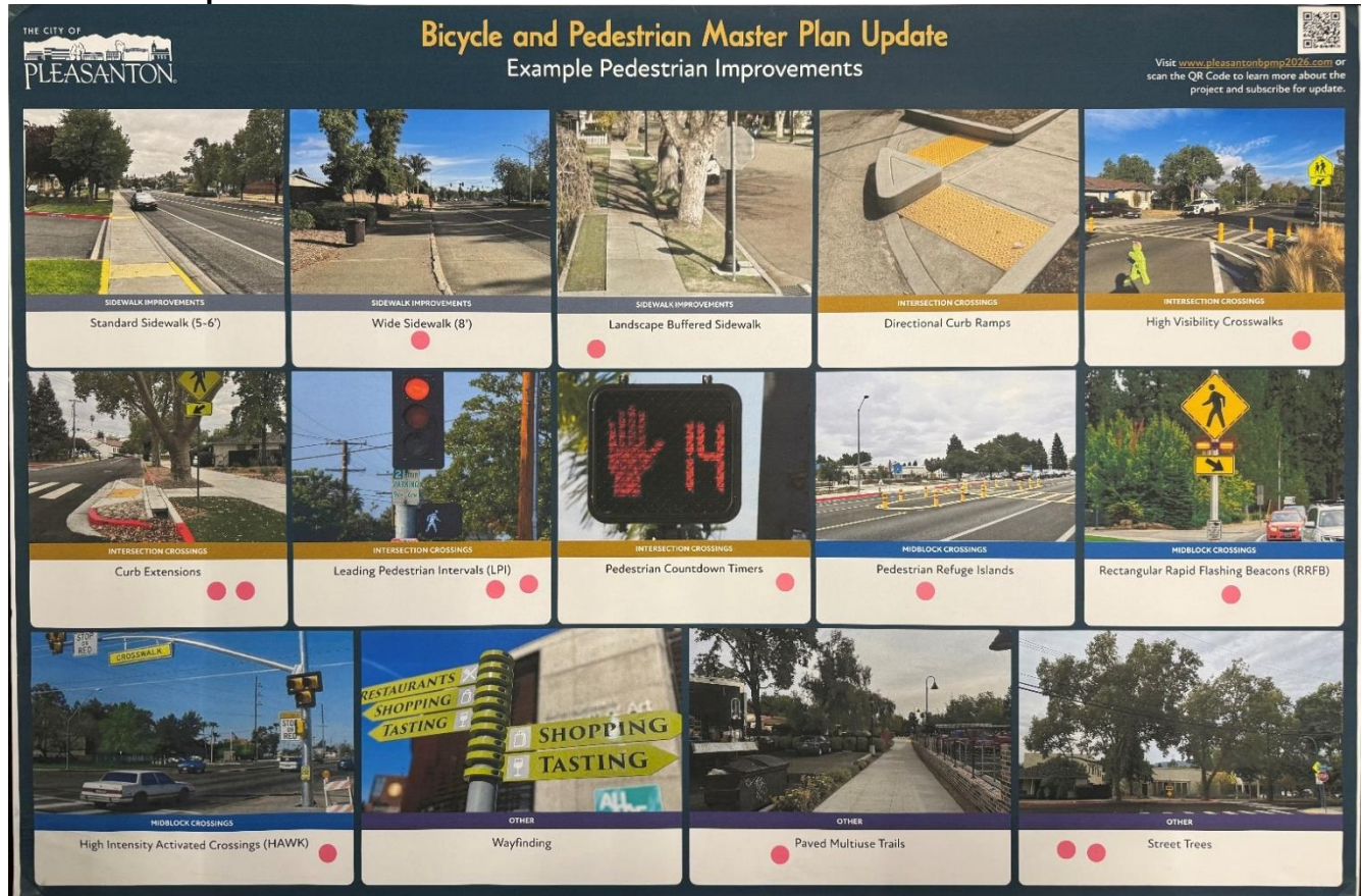
Figure 5 Pedestrian Improvements Board
