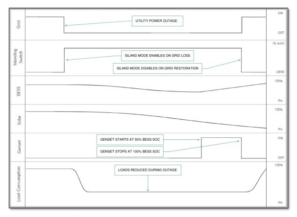
Figure 14. DER Resilience Scenario Timing Diagram
