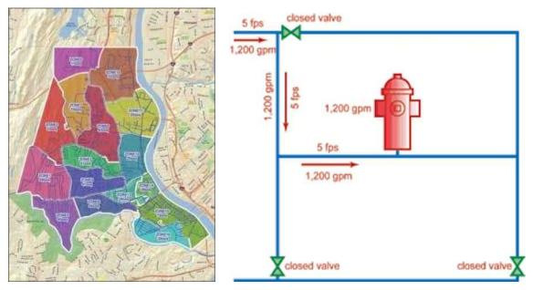
Figure 2. Examples of Unidirectional Flushing Program Zones
