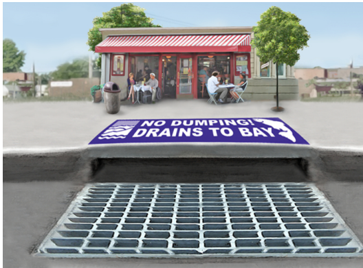
Storm Drain: An outdoor drain that flows directly to creeks and the Bay.
