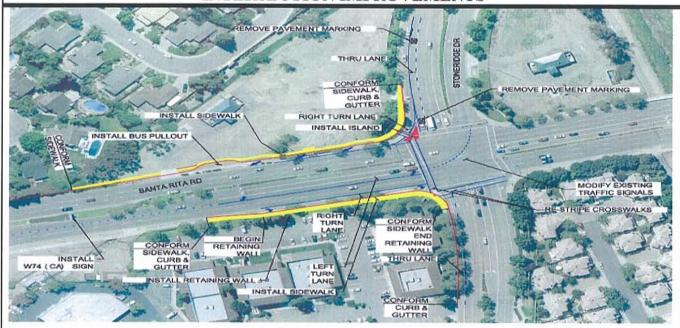
**PROJECT DESCRIPTION**: This project involves converting the second eastbound right lane to a through lane, converting the eastbound right turn lane to a free right turn lane, constructing a northbound right turn lane, converting the northbound through lane to a third northbound left turn lane, and installing a bus pullout on southbound Santa Rita Road.
