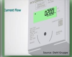
The "flow rate" screen is pictured above. The flow rate will change continuously depending on how much water is used or leaking.
