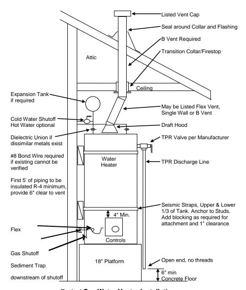
**Typical Gas Water Heater Installation**
